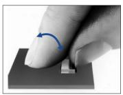
2) Rotate down the actuator until firmly closed. NOTE: The FPC must be fully inserted in the connector. If not fully inserted, the actuator will not close properly. Should this be the case, lift up the actuator (per Step 2 below) and repeat the process (starting with Step 1 above)
