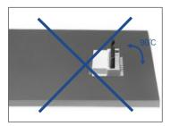
3) Assure that the FPC is fully inserted parallel to mounting surface, with the exposed conductive traces facing down.
