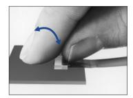
1) Do not apply excessive force or use any type of tool to operate the actuator.
