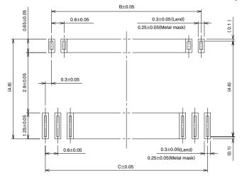
Recommended metal mask thickness: t = 0.1 mm
